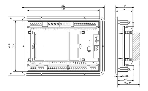
**Note:** The final depth of the controller depends on the selected extension module - it can vary between 41 and 56 mm. Mind also a size of connector and cables (e.g. in case of RS232 connector add about another 60 mm for standard RS232 connector and cable).
